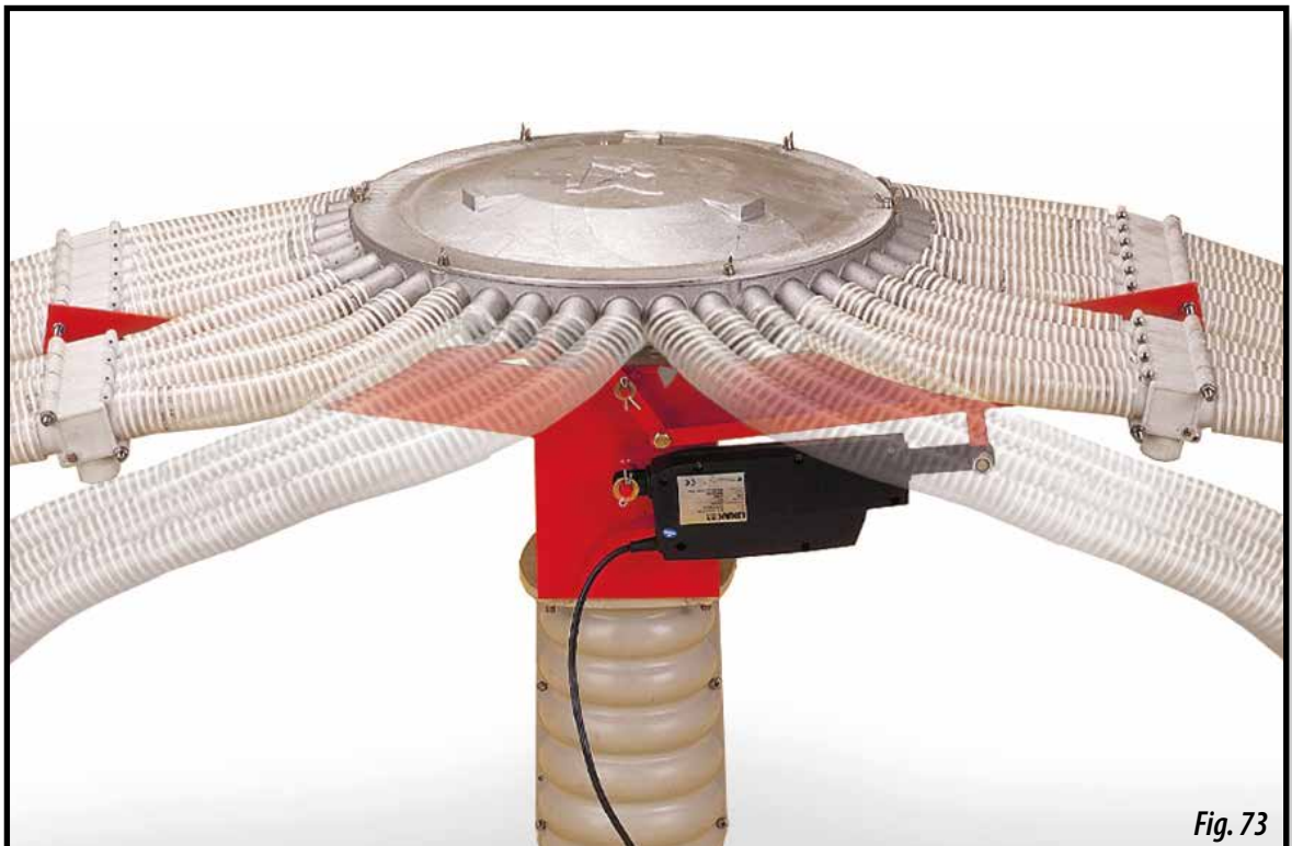
Seed hoses closing system in folding parts / tramlines
