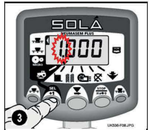
Figure 8: View Wing Width
