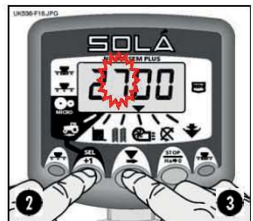
Figure 16: Low speed alarm threshold
