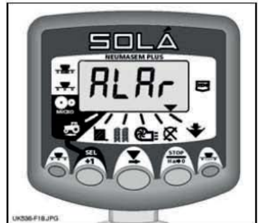
Figure 18: Hopper Low Alarm
