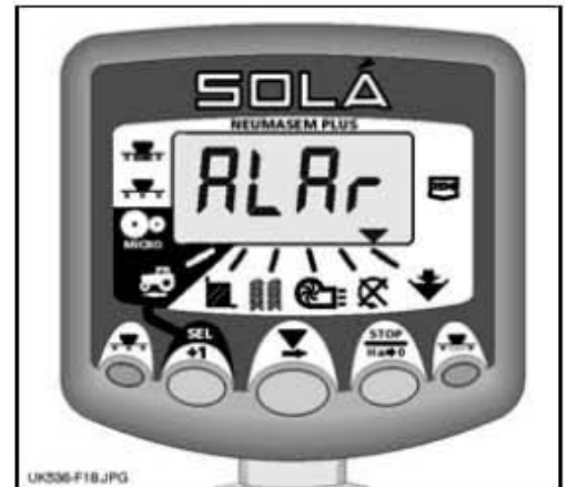
Figure 18: Hopper Low Alarm
