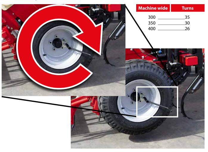
You must turn the wheel uniformly using the crank at approximately one revolution per second, depending on the land's characteristics, tyre's manufacturer or tyre pressure. For this reason it is highly recommended to perform a field test as described in this manual (4.5).
