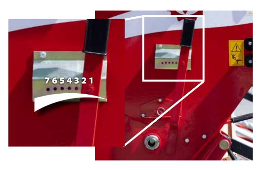
The base flap lever (placed on the left side of the hopper) has 7 positions
