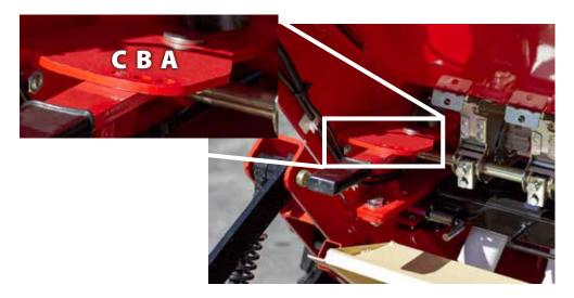
Move the lever to switch between narrow and wide position in the seed wheel
