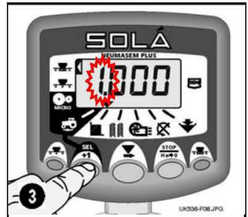
Figure 8: View Wing Width
