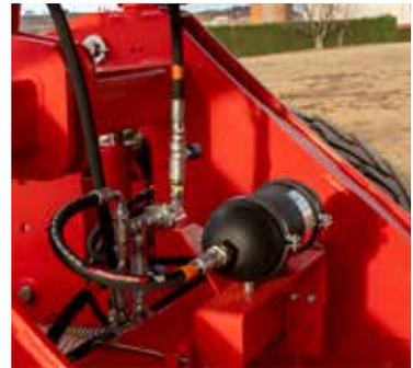
3-pt hitch hydraulic damping for safe transport.
