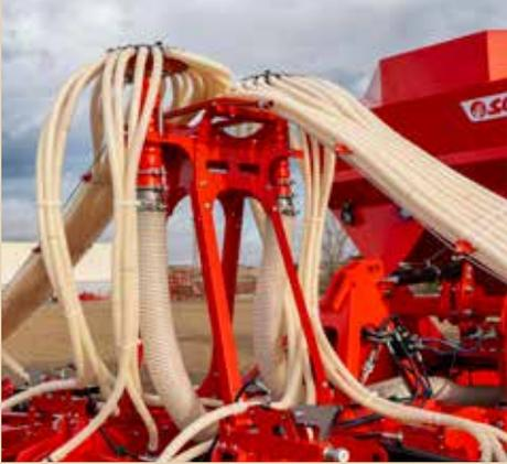
Double distribution head for half-machine shutt-off
