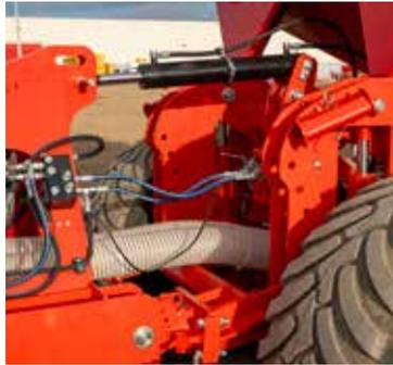
Rear three-point hitch with 7,800 kg lifting capacity.
