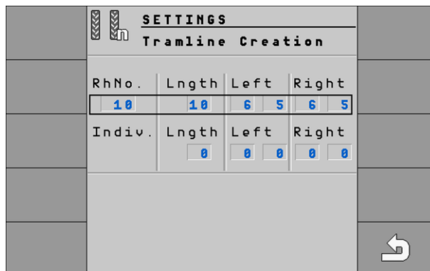
“Settings / Tramline” screen for a seeder
