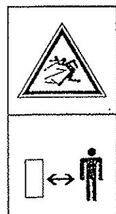
Stay away of the fertilizer spreader. Fertilizer grains impact can cause a serious lesions.
