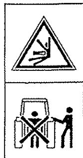
Stay away of the tractor back part during the coupling operation.
