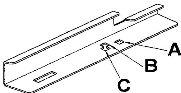
Left blade ( it must be fitted on the disc of the left side in starting sense)
