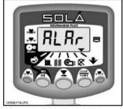
Figure 18: Hopper Low Alarm
