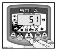
Figure 17: Distribution Shaft speed
