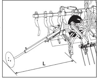
working width seed drill - track gauge wheels tractor + width of the row
