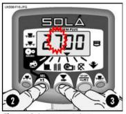
Figure 16: Low speed alarm threshold
