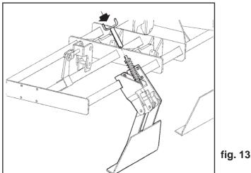
The leveler must trail the land but avoiding that the land running over the plate. To erase the seed drill marks, we can fit the track erasers. We have to adjust them.
