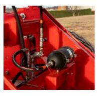
3-pt hitch hydraulic damping for safe transport.
