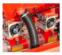
Stainless steel metering units with easy access for maintenance and quick-emptying system.
