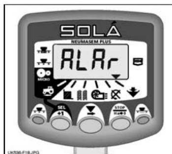
Figure 18: Hopper Low Alarm
