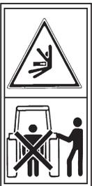
Stay away of the tractor back part during the coupling operation, during the coupling manoeuvre. **Danger of serious lesions.**
