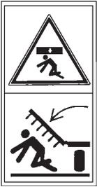
Do not place under the sowing equipment or under swinging areas.
