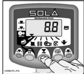
Figure 1: Display Forward Speed
