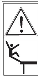
Do not ride on the seed drill stairs when the machine is working. **Danger of serious lesions.**
