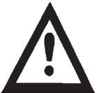
Be extremely carefully actuate the tractor power take-off. ABRUPT STARTS COULD CAUSE IMPORTANT DAMAGES IN THE SEED DRILL.
