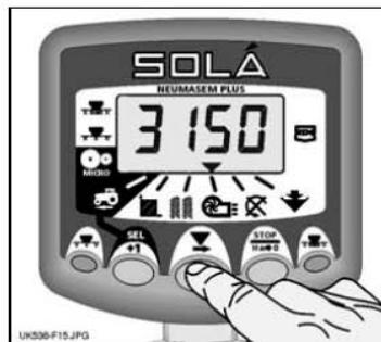
Figure 15: Display Fan Speed
