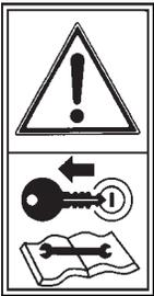
Stop the tractor engine and avoid its start during the maintenance or repairing works in the seed drill.
