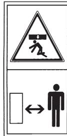
If you are working under the machine, it is very important to assure it, to avoid its collapse. **Danger of serious lesions.**
