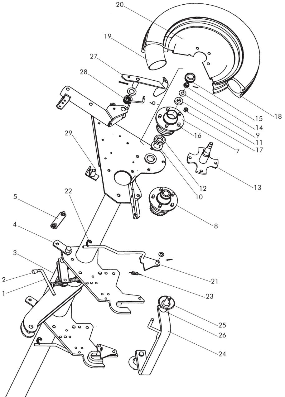
*9.2 CHASSIS ET ROUES DU SEMOIR SIMPLE ET DU SEMOIR COMBINE*
