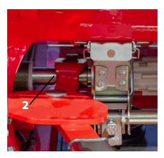
The central adjuster spindle. Use solid calcium grease (3)
