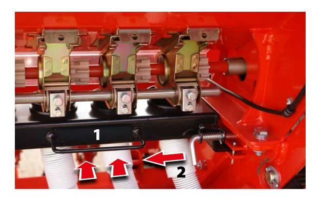
SECOND: slide the plate from the transport position and place it under the dispensers.
