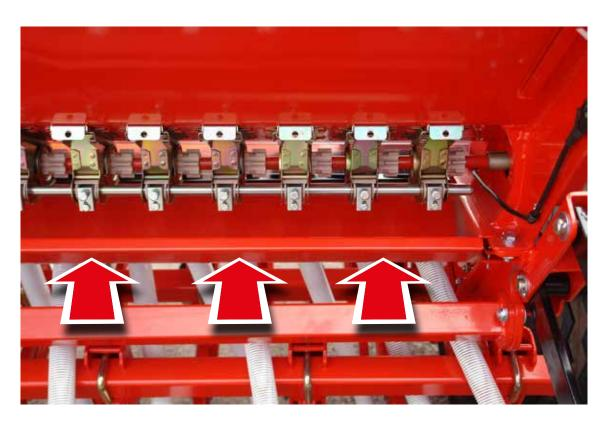
**THIRD:** Raise the seed drill using the tractor until the wheels can turn freel. Place the calibration crank in the bolt on right wheel and turn it clockwise until seeds start to fall onto the calibration cup. At this moment, stop turning, put these seeds back inside the hopper and start turning the crank again to perform the real turns of the test.
