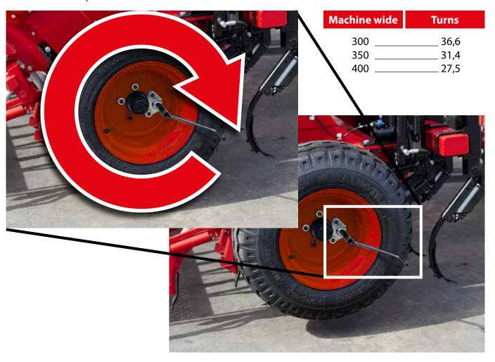
You must turn the wheel uniformly using the crank at approximately one revolution per second, depending on the land's characteristics, tyre's manufacturer or tyre pressure. For this reason it is highly recommended to perform a field test as described in this manual (see section 5.5).
