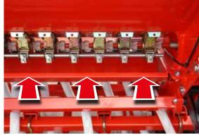
THIRD: place the lever in its place on the left wheels and five some clockwise turns to the driving wheel, until some seed is delivered. Collect up the fertilizer and return it to the hopper and and give the turns as follows:
