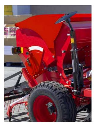
In order to transport the machine, it is essential to fold the track markers so they stay in a vertical position and pin them to the transport bracket using a lynch pin. This will prevent them from lowering during transit.
