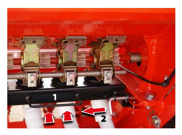
**SECOND:** Pull the calibration cup upwards out of their holders and place it under the seed wheels.
