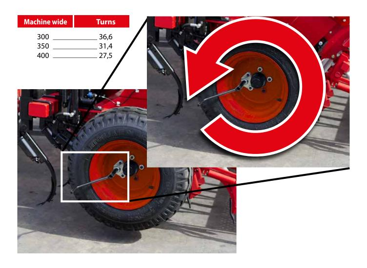
The fertilizer collected, multiplied by 40, are the fertilizer kgs per hectare that the machine will distribute with the lever in the sector choosed. It is very important to do a precision test with the fertilizer, to verify the fiability level of the dosage table.
