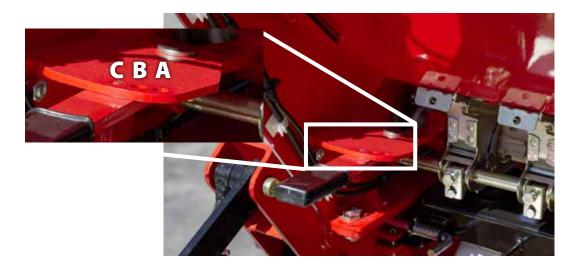
Move the lever to switch between narrow and wide position in the seed wheel
