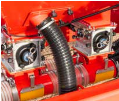
Stainless steel metering units with easy access for maintenance and quick-emptying system.
