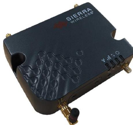
If you want to use the NAV-900 with CenterPoint VRS, you must always also connect an RV55 modem to the receiver. In addition to the modem and an additional connector cable (item no.: 3038990027), you also always need a SIM card, which you must insert in the modem.
