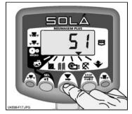
Figure 17: Distribution Shaft speed
