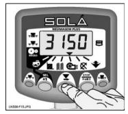
Figure 15: Display Fan Speed
