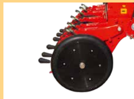
Roue tasseuse en V de 1" ou 2" réglable. "V" shaped pressing wheel of 1" or 2" with adjustable pressure and tilting.
