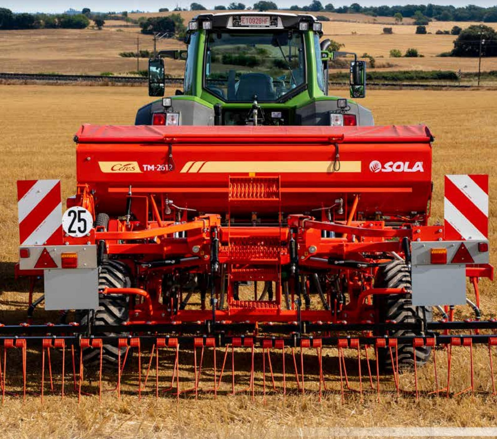
Folding telescopic system of the seeding equipment. From 3m. in transport position to 4m. in working position.
