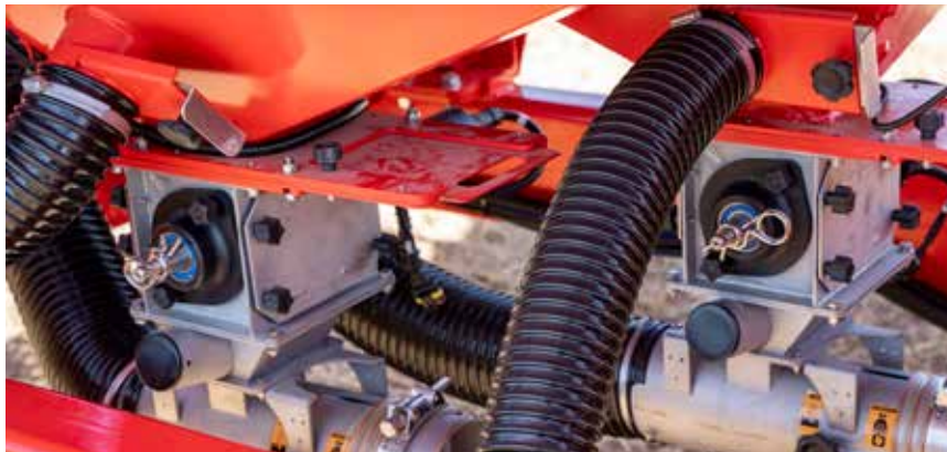
Stainless steel metering units with easy access for maintenance and quick emptying system.
