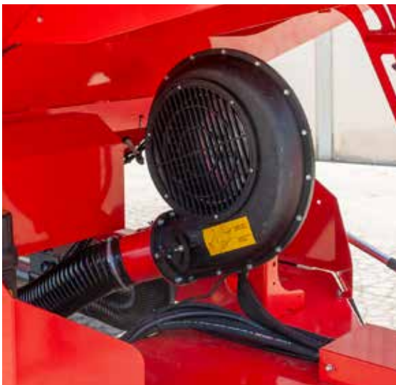
Highly efficient turbine with hydraulic drive.
