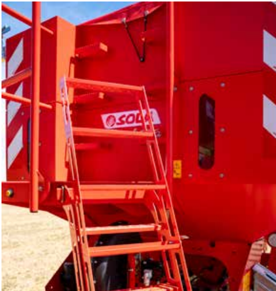
Platform access ladder. Control windows.
