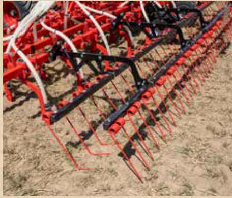
Easily adjustable double spring harrow.
