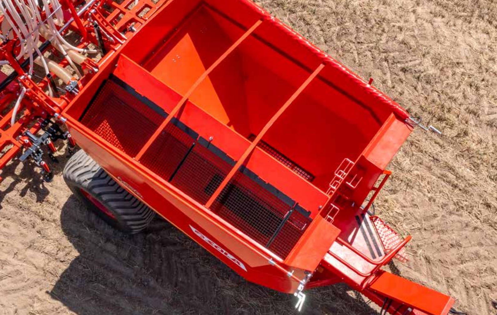
Large capacity hopper divided 60/40 for seed and fertiliser.
