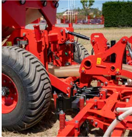
Three-point linkage with 5,600 or 7,800 kg lifting capacity
