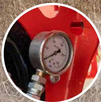
Pressure gauge of the turbine hydraulic system.
