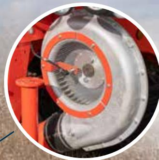
Hydraulic drive turbine built in aluminum body.
