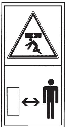
Danger of crushing when working under the machine. Secure it to avoid accidental falling.
