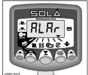
Figure 18: Hopper Low Alarm
