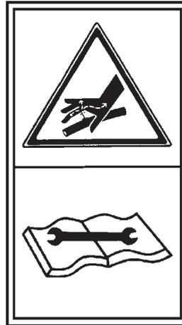
Possibility of penetration by hydraulic fluid. Keep in good condition the h y d r a u l i c hosepipes.
