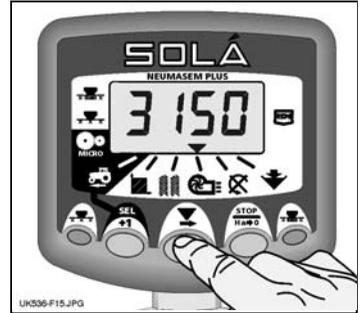
Figure 15: Display Fan Speed
