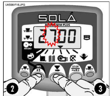
Figure 16: Low speed alarm threshold
