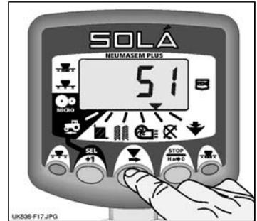
Figure 17: Distribution Shaft speed
