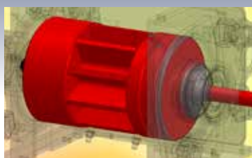
Volumetric metering unit with electric drive with interchangeable modular rollers.
