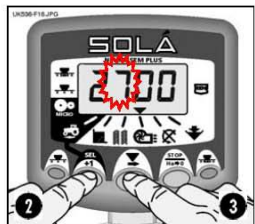
Figure 16: Low speed alarm threshold
