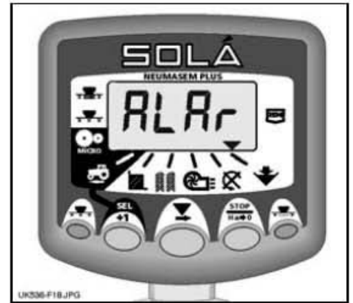
Figure 18: Hopper Low Alarm
