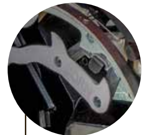
Self adjusting singulator
