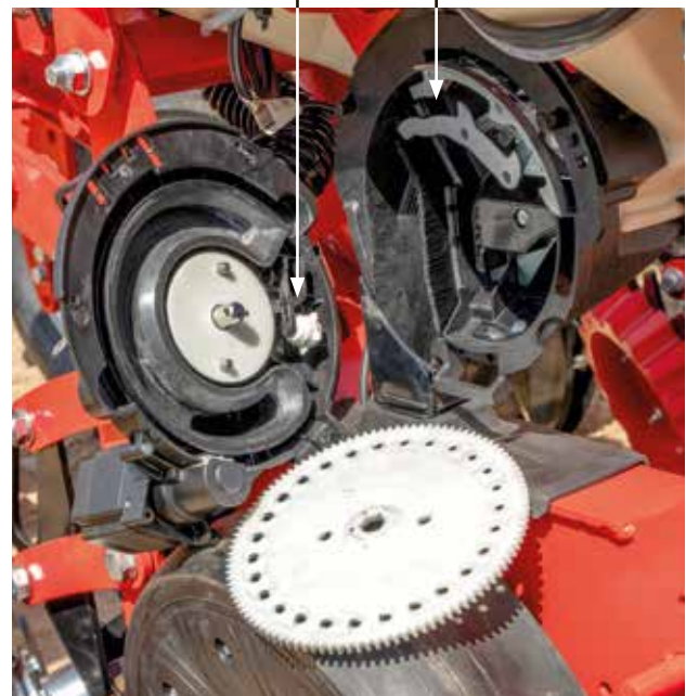
Self adjusting singulator
